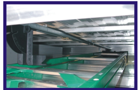
Raise the foot of the ladder & secure it to the catch bracket.
