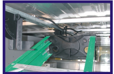
Slide the ladder forward along the rail.
