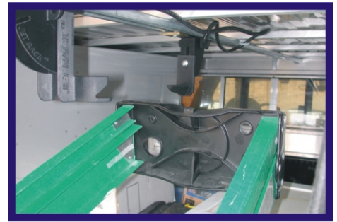
Hook the ladder top onto the receiving pin.
